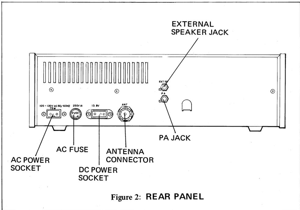
Your SSB-M6 is a full 40 channel AM/SSB-Base/Mobile Citizens Band Transceiver skillfully constructed by employing the latest frequency synthesizing technology. The Model M-6 will be operated from both AC and DC power sources. The transceiver incorporates many other features such as a Clarifier control for clearer reception, an NB switch for quiet reception, Tone Switch for desirable tonal quality when receiving, RF GAIN control and easy-to-read L.E.D. channel digital read-out.
