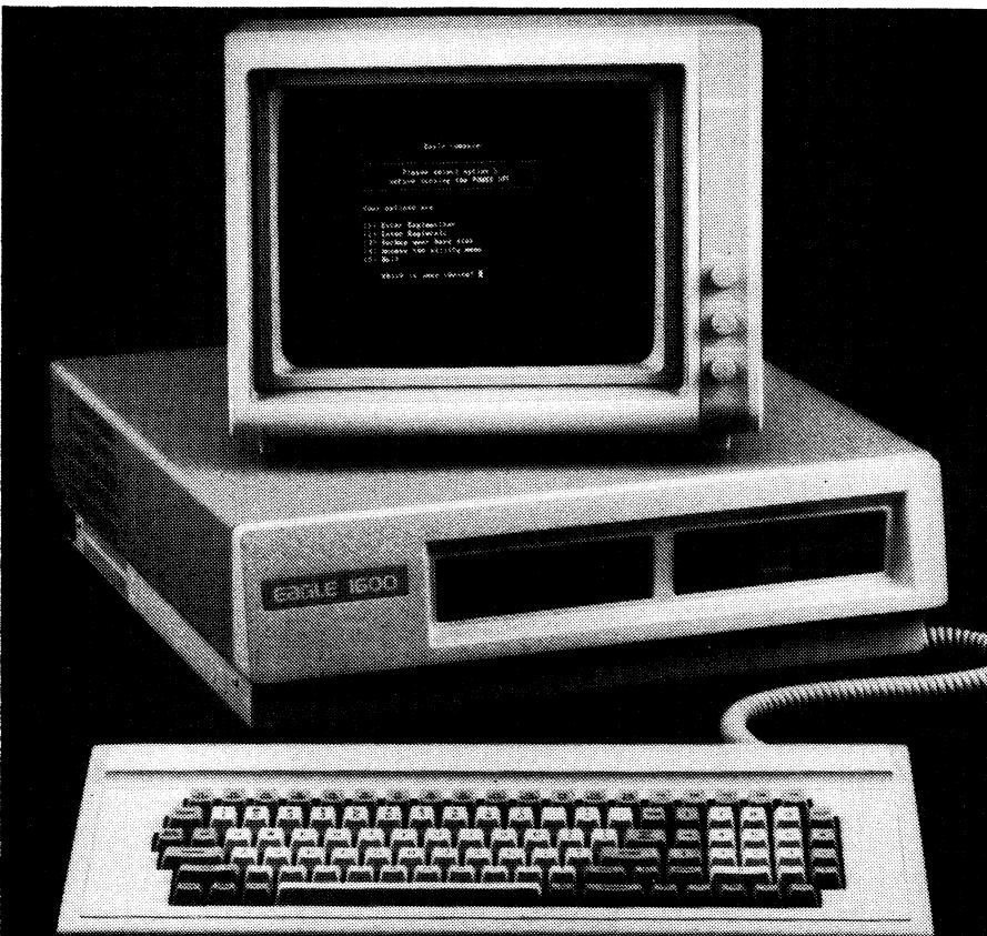
The Eagle 1600, distributed in Australia by Scomco Pty Ltd, was introduced at the DATA '83 exhibition. Features include an 8MHz 8086 processor and 10MB hard disk.
