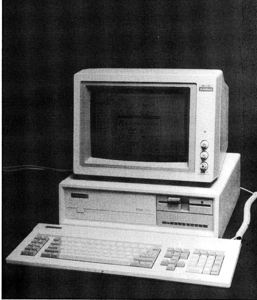
The standard Multitech PC-700 comes with two 360K floppy drives. This machine was fitted with the optional 20M hard disc drive.
