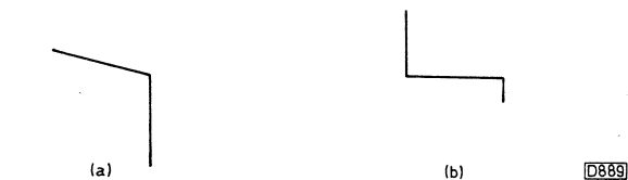
Fig. 14: Tests on LEDs. (a) Waveform for a small LED. (b) Waveform from a seven-segment LED.
