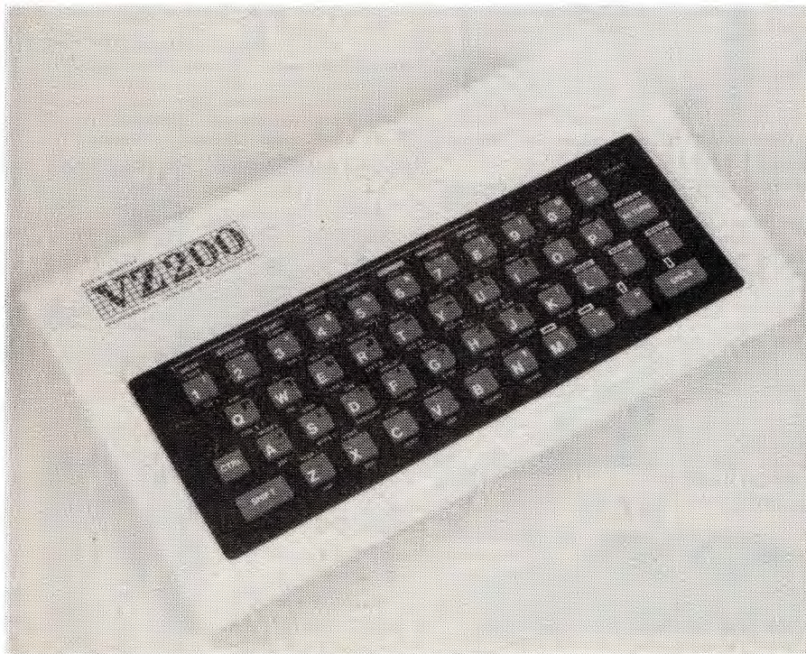
The VZ-200 computer. The keyboard has 45 moving keys with audible feedback.
