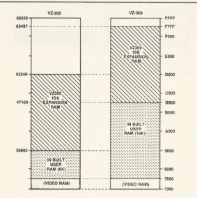
Figure 1. The memory maps for the VZ-200 and VZ-300. Note how their internal and expansion RAMs cover different address ranges.
