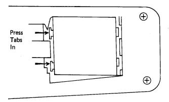
Special Note: Never leave weak or dead batteries in the unit. Do not store the unit with batteries inside. When tones become weak and/or lights slow down, replace with fresh Alkaline batteries.
