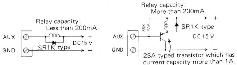
Relay will operate when scanning stops.
