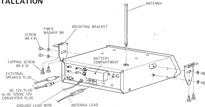
**NOTES: BATTERY INSTALLATION:** Before turning your SX-200 on make certain that you install the two SIZE AA BATTERIES supplied in the battery housing on the rear panel being careful to put them in with the correct polarity (Polarity is marked on base of plastic holder.) The batteries are used for memory backup.
