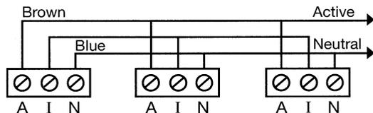
Connecting the switch wire terminal in any other way to that shown in this instruction may result in damage to the alarm, failure to operate or an electrical shock hazard. It will also void the warranty.
