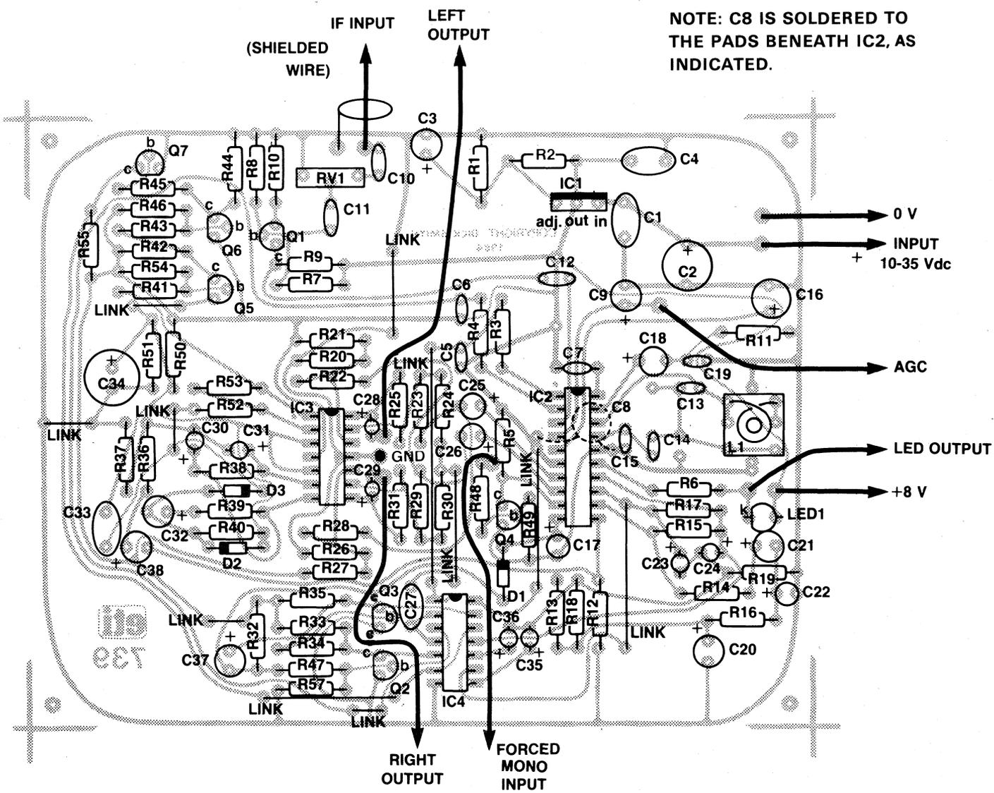
NOTE: C8 IS SOLDERED TO THE PADS BENEATH IC2, AS INDICATED.
