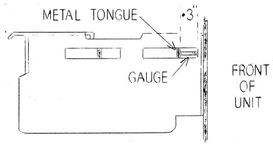
Turn the tuning control until the metal tongue in the slot touches the .3" gauge.
