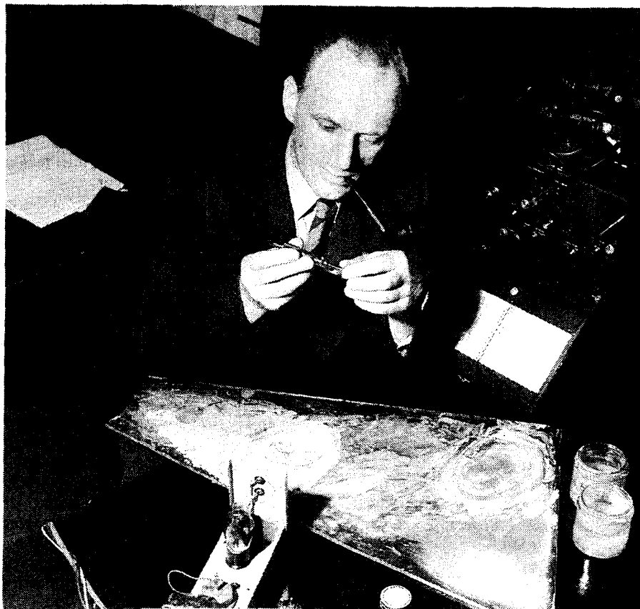
Complete with pipe and micrometer, John is pictured here with his crystal-grinding paraphenalia spread out on the table: frequency meter (top right), a slab of rigid very flat glass and (foreground) his test oscillator. In those days, crystals were large enough to handle – gingerly! (Courtesy Dr Alice Moyle)
