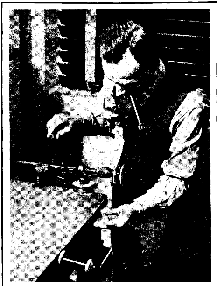
John Moyle in a characteristic pose, pipe in mouth and concentrating on the job in hand — here the winding of an inductor for a loudspeaker crossover network.
