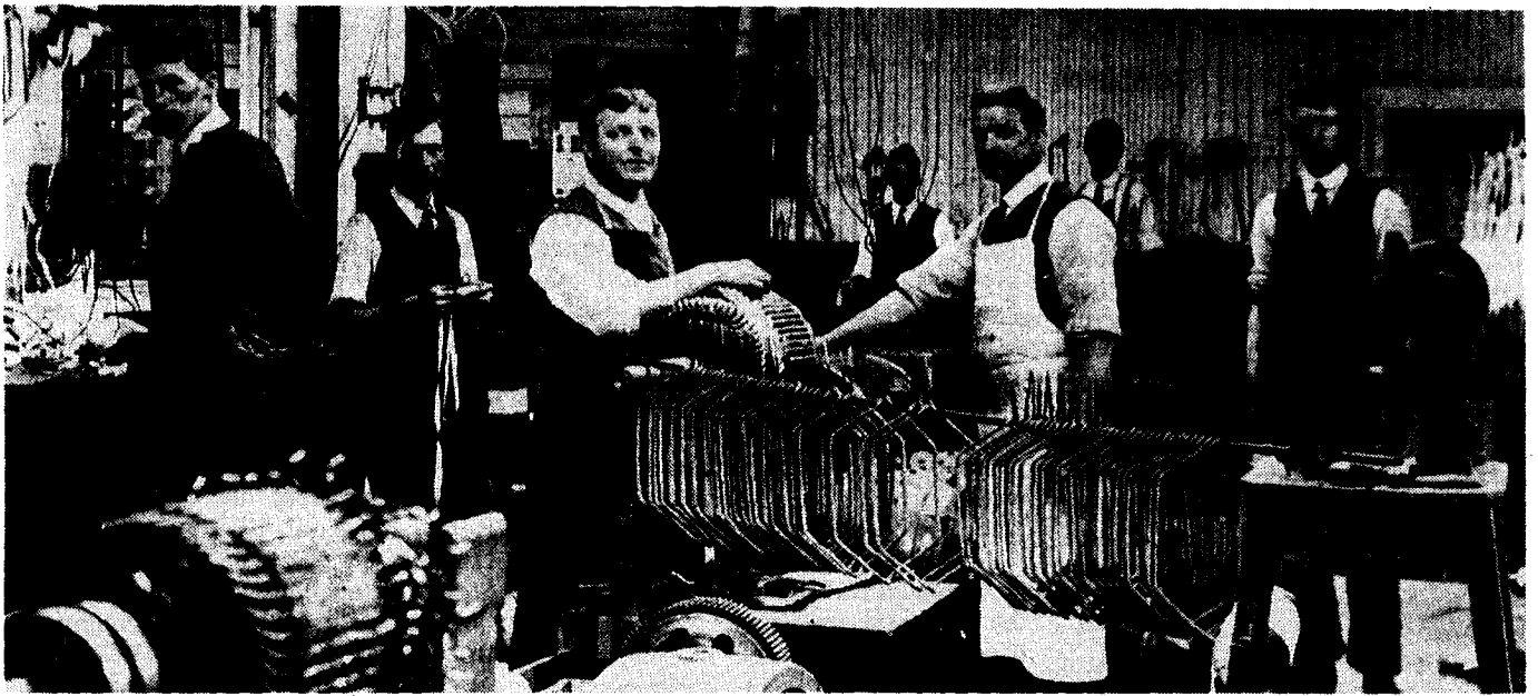
Another view inside the radio factory in 1912, this time showing the motor/alternator winding and fabrication area. Note the windings hung up to dry, after varnishing.
