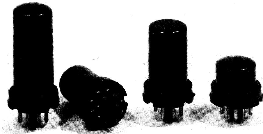
**Examples of the first 'all metal' 8-pin octal based valves which first appeared in America around 1935. Later octal valves had a glass envelope.**
