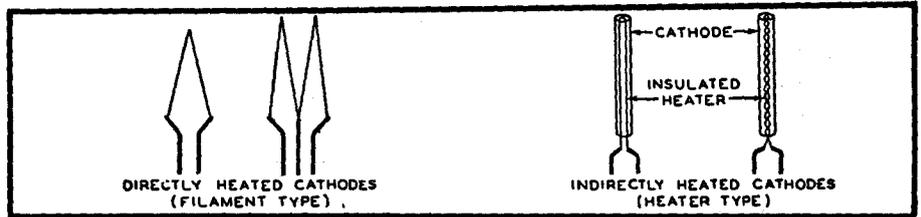
**Fig.3:** To minimise current drain, battery valves normally use a directly heated coated filament (left). But most mains powered valves used an indirectly heated cathode (right), to minimise hum injection into the signal path.
