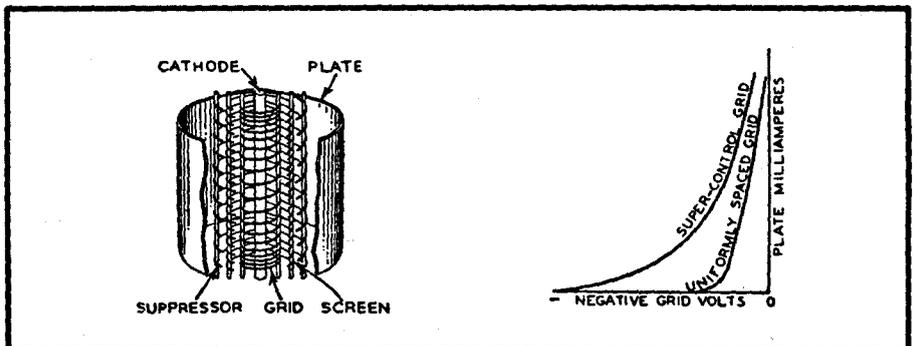
**Fig.5:** At left is the electrode structure inside a pentode valve. The grid winding pitch was normally uniform, but a variable gain or 'super-control' characteristic (right) was achieved by varying the control grid pitch over its length, as shown.
