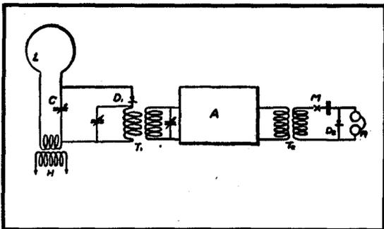
**Fig.1: From Armstrong's own paper published in Australia in September 1921, the basic concept of a superhet receiver. Early superhets commonly used loop aerials to minimise objectionable signal radiation from their heterodyne oscillator.**
