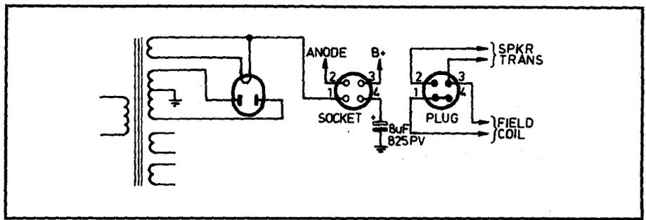
**Fig.5:** Wiring a loudspeaker socket and plug as shown above could protect the first filter capacitor from damage in the event of a receiver being switched on without the loudspeaker being plugged in.
