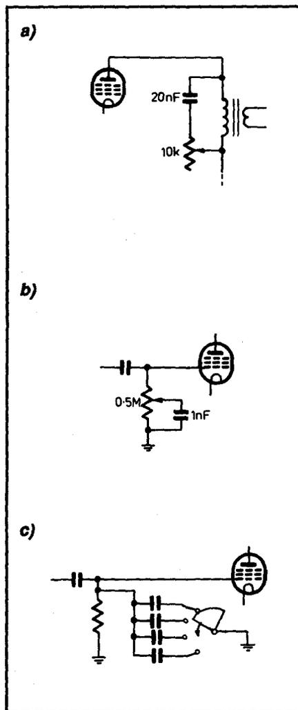
**Fig.4: Three typical methods of providing a top-cut tone control in the early 1930's.**
