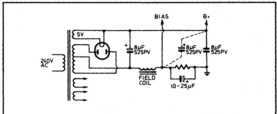
**Fig.6:** For reasons best known to themselves, some designers included the loudspeaker field winding, as well as the back-bias resistor in the negative supply lead. It placed about -200V on the exposed shell of the first can type electrolytic!
