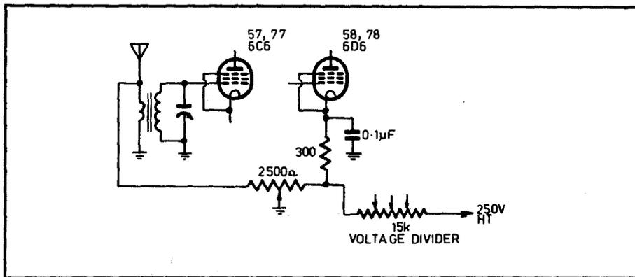
**Fig.2:** A method of eliminating the local/distant switch, by so arranging the gain control that it shorts the antenna to earth in the fully anti-clockwise setting.
