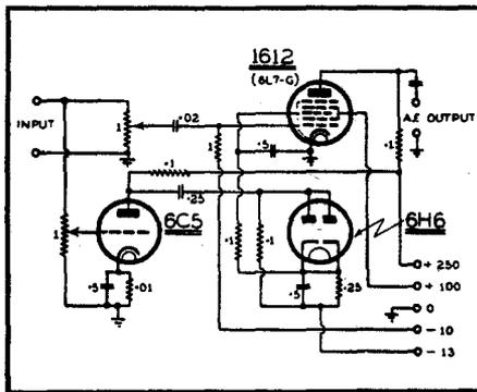
**Fig.4: Basic automatic volume expansion circuit from the 'Radlotron Designer's Handbook, 3rd edition, p.74**
