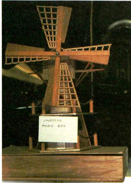
Before the phonograph — a novelty music box. A spring driven mechanism rotates the 'sails' while also driving the spiked roller which plays a tune by plucking 'reeds'.
