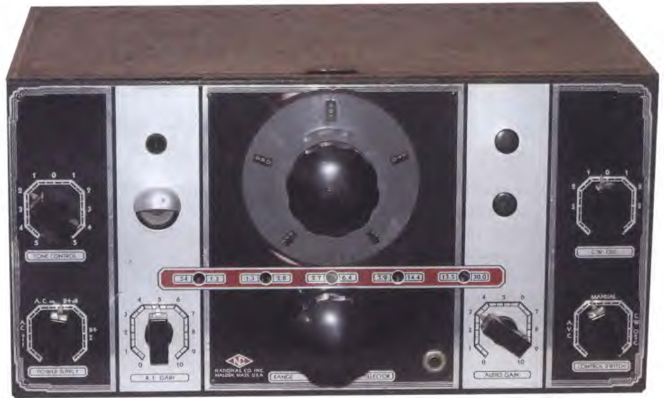
Fig. 3: The NC-100 receiver, with the very familiar tuning knob.
