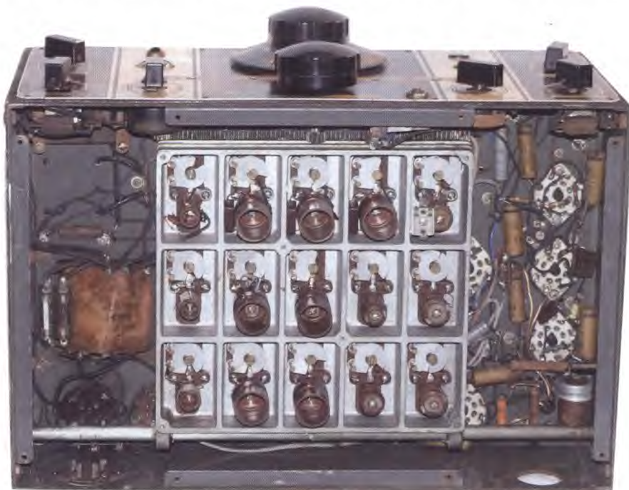
Fig. 4: The NC-100's unusual coil switching arrangement.
