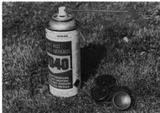
A spray with WD40 or similar penetrating fluid often helps loosen stubborn control knobs. The knobs can then be cleaned with a stiff brush and detergent.
