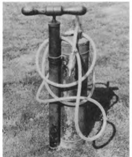
Compressed air is a handy aid when cleaning old radio chassis. This home-made outfit was put together for just a few dollars.
