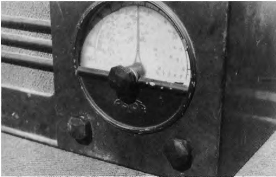
The knobs on this old Astor seemed to be welded on and at least four attempts were made to remove them before they finally yielded.
