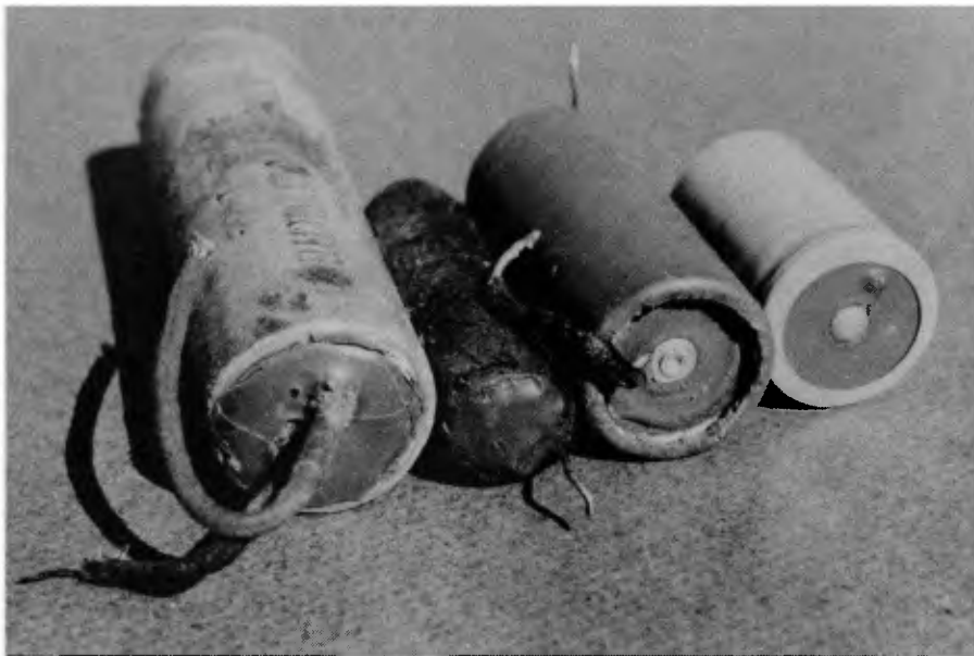
Old electrolytic capacitors are a common source of serious trouble in vintage radios. The replacement of all electrolytics during restoration can save a lot of hassles later on.
