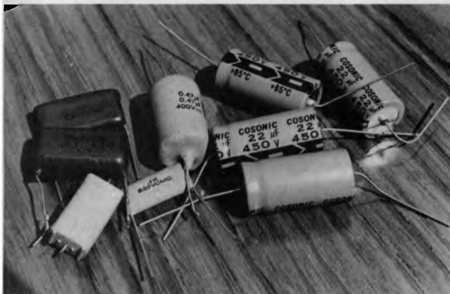
Many of the capacitors used in valve radios are high voltage types. Always make sure that replacement capacitors have an adequate voltage rating.
