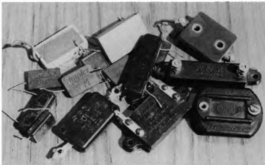
A selection of old mica capacitors. These capacitors are very reliable and seldom require replacement with more modern types.
