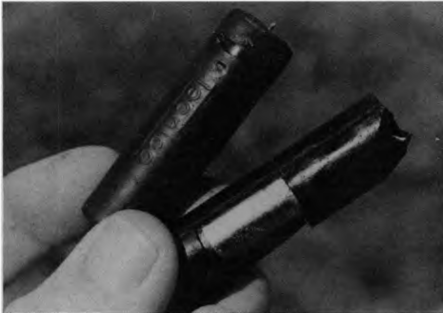
A couple of typical paper capacitors — cracked, troublesome and quite unreliable.
