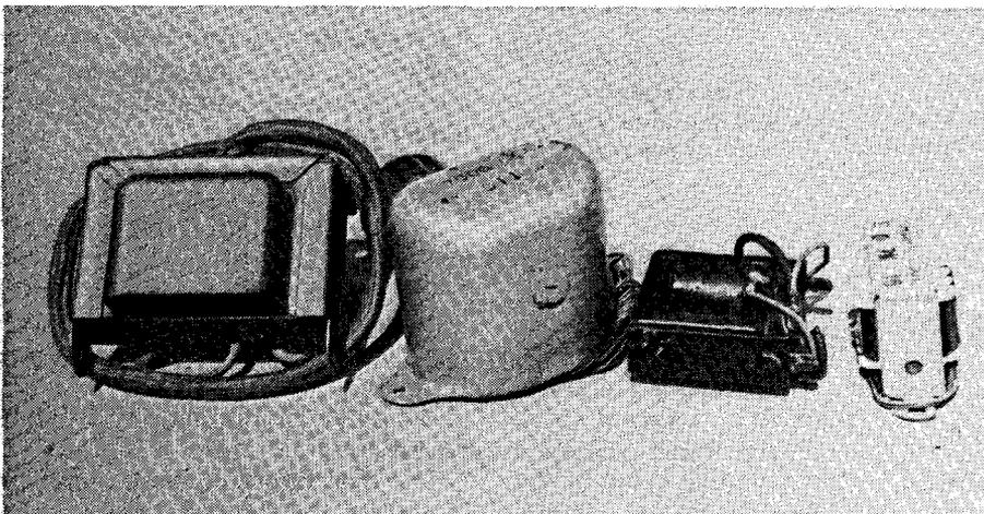
Loudspeaker transformers can be unreliable so it's always a good idea to have a good stock of spares. In particular, you should always save the speaker transformer if you junk a set, along with any other parts that might prove useful.
