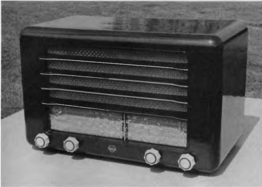
This stylish old receiver was made by Mullard. Its Bakelite cabinet was in excellent condition and has been restored so that it now looks brand new.
