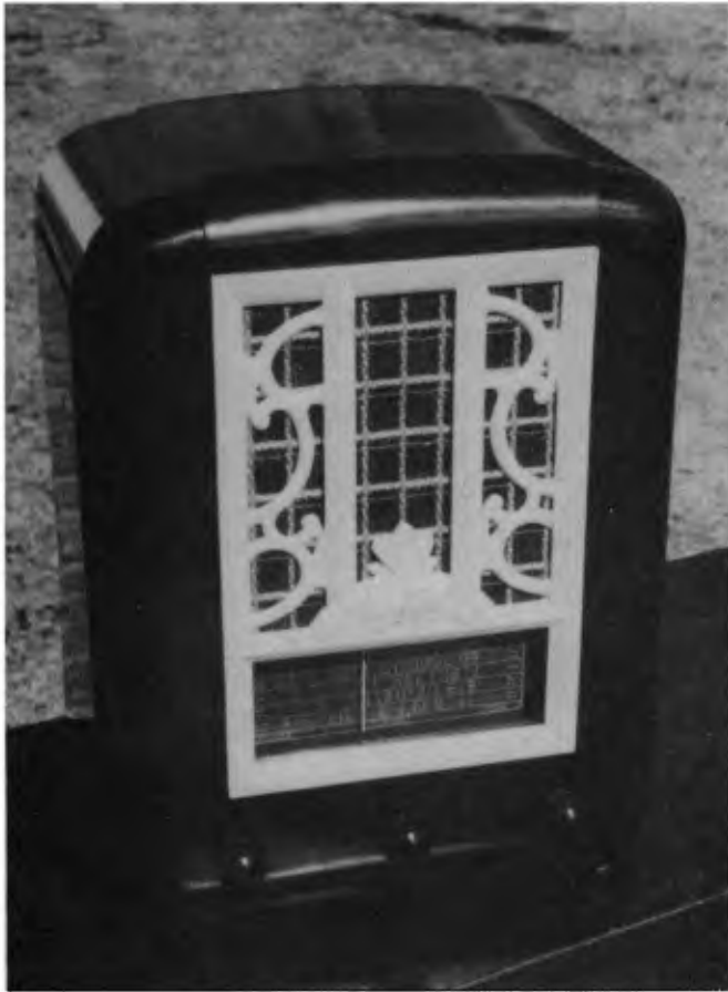
The cabinet of this 1937 model Airzone was cracked in three places due to rough treatment but was repaired satisfactorily using super glue. These receivers used a rather complicated dial mechanism.
