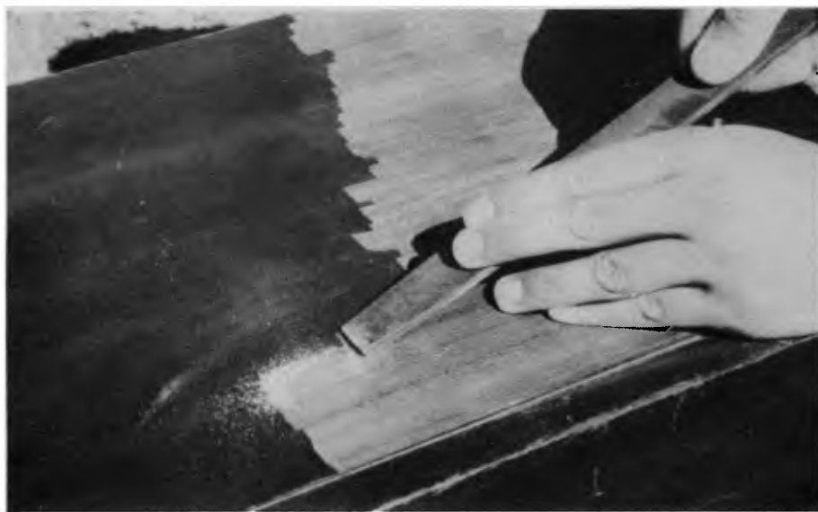
An old flat file makes a handy varnish scraper but care must be taken not to dig the corners into the timber. If the lacquer is difficult to scrape off, you may have to resort to using paint stripper.
