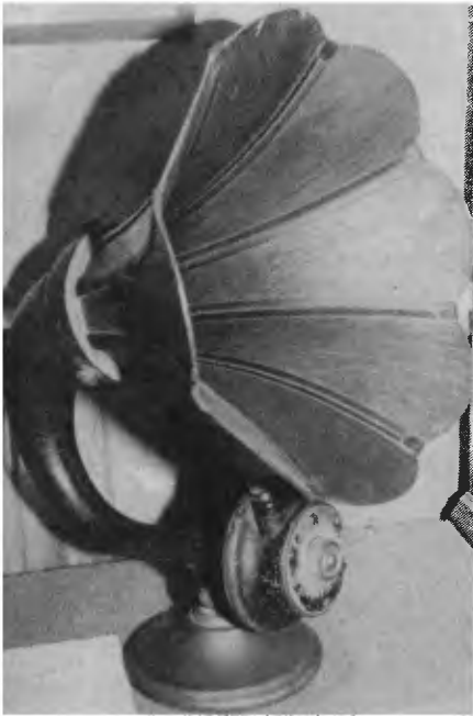
Amplions with a timber flare would be the ultimate collectors' items as far as horn speakers are concerned. (Photo courtesy Orpheus Radio Museum, Ballarat).
