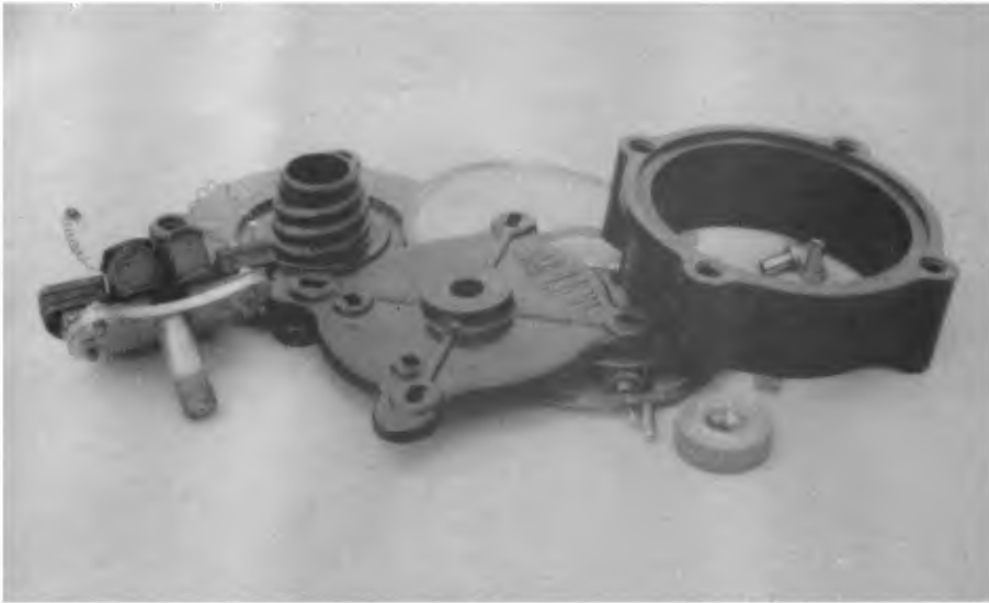
These parts are all from a dismantled Amplion driver. The body appears to be made of moulded ebonite (hard rubber). Note the pole pieces at left.
