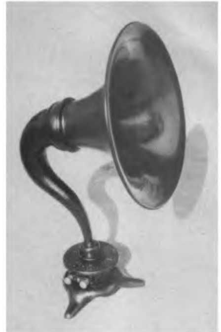
This English-made Amplion horn speaker is the best performer in the author's collection. Notice the two connecting terminals on the base.
