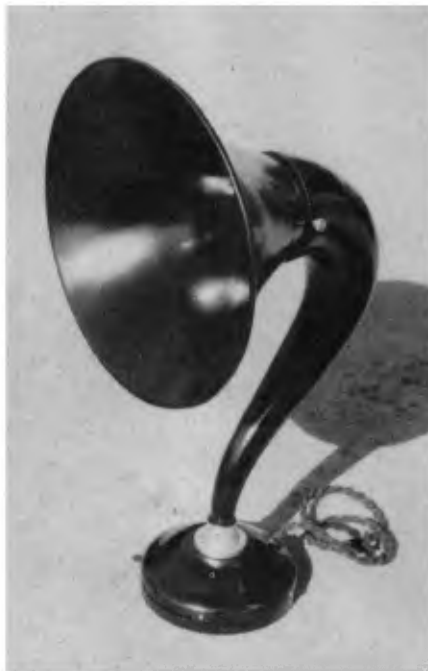
This Sterling "Baby" horn speaker is one of the few in my collection that didn't require rewinding.
