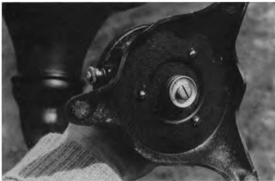
Horn speakers have an adjustment which varies the spacing between the pole pieces and the diaphragm. This adjustment affects both the tone and the volume.
