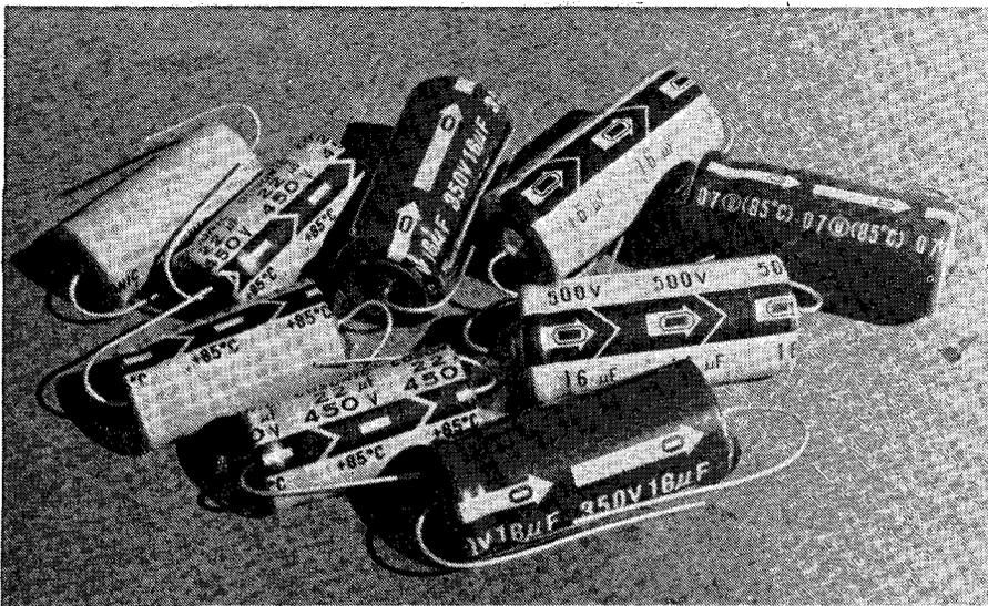
**Electrolytic capacitors are capable of storing a substantial electric charge and should be discharged as a matter of course after switching a set off. Remember that switching off at the power point doesn't always eliminate all of the nasties.**
