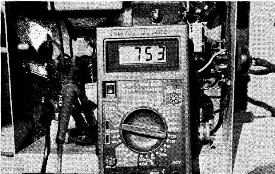
**The digital multimeter says it all — don't underestimate the dangers when working on valve radios. In this case, the meter is measuring the AC voltage across the anodes of a rectifier valve.**
