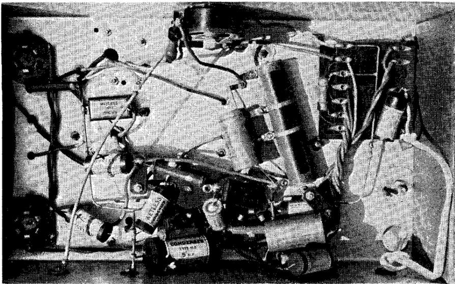
There are numerous high voltage components underneath a valve chassis so don't go poking around indiscriminately. Safe work habits need to be adopted at all times when working on valve radios, otherwise you could get a nasty shock.
