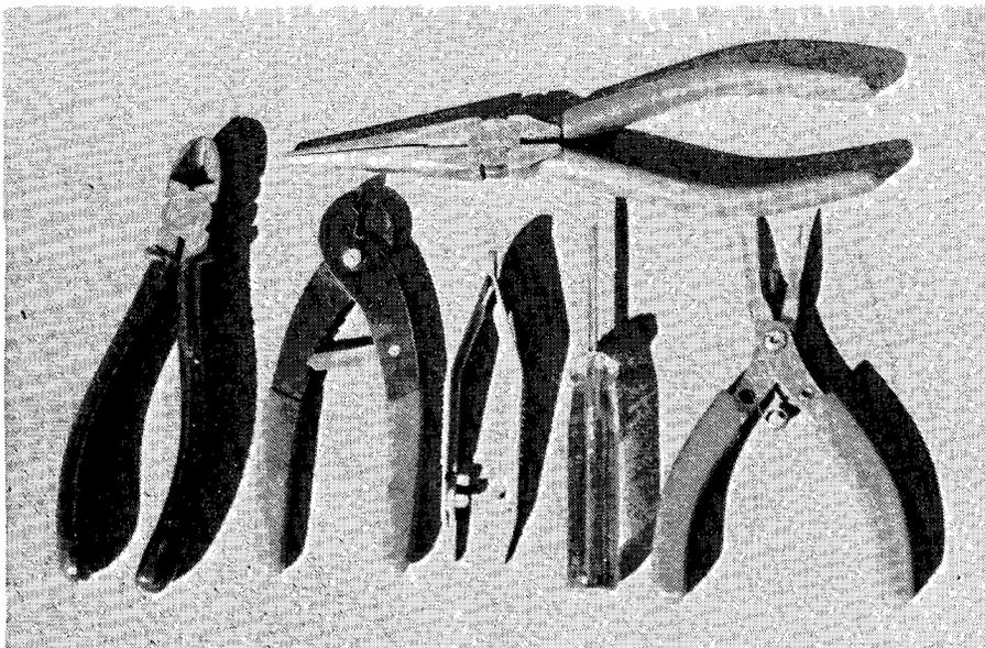
**Electrical hand tools require insulated handles — particularly when working on high voltage valve equipment. Replace the tool if the insulation becomes worn or perishes.**
