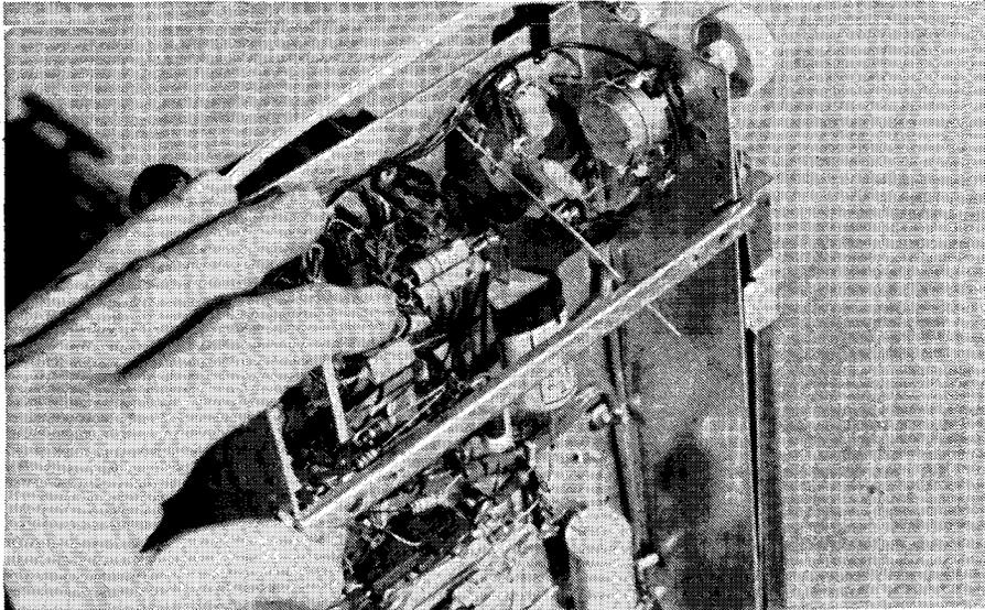
**Keep that free hand in your pocket when working on an upturned chassis. Using a finger as the path of least resistance can have fatal consequences.**
