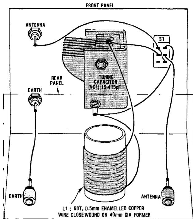
**Fig.2: here's how to wire up a practical wave trap with IN/OUT switching. Use one section of a 2 or 3-gang tuning capacitor if that's what you have available.**
