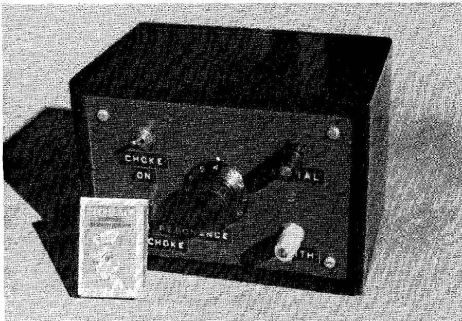
This is the author's wave trap. It need not have been so large but the box was available — it previously housed a crystal set. A much smaller unit could be built using more modern components.
