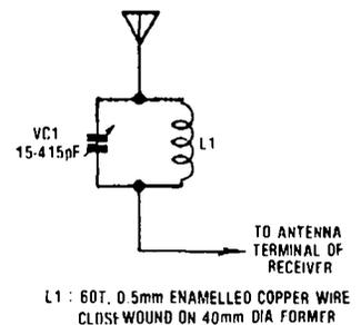
Fig.1: a wave trap consists of a tuned circuit in series with the aerial input.
