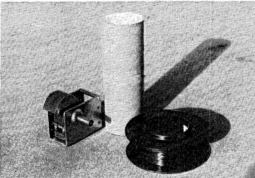
A basic wave trap is nothing more than a tuned circuit made up of a coil and a variable capacitor. The capacitor need not be a single gang unit. Instead, you can use a 2 or 3-gang unit salvaged from a derelict radio.
