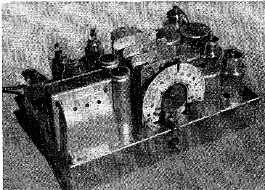
This superhet receiver has an intermediate frequency of 175kHz. A wave trap helps to reduce the number and intensity of the heterodyne whistles that occur when such a set is operated in close proximity to a powerful local station.
