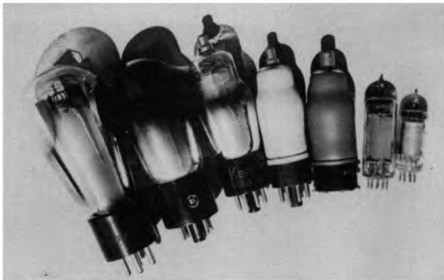
Radio valves became progressively smaller as time progressed. Whatever their age, all newly acquired secondhand valves should be checked in a valve tester or in a working receiver to determine their condition.
