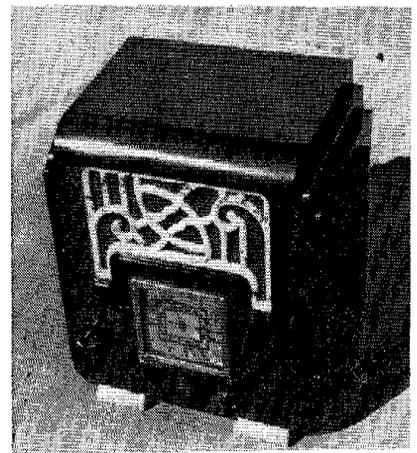
The valve complement of this old Radiolette was common for many 1936 receivers. The line-up was 80, 6A7, 6D6, 6B7 and 42.
