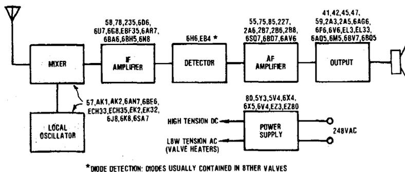
Fig. 1: this diagram lists most of the valves likely to be encountered in the average Australian-built receiver and shows where they are used. About 60 different types just about covers everything.
