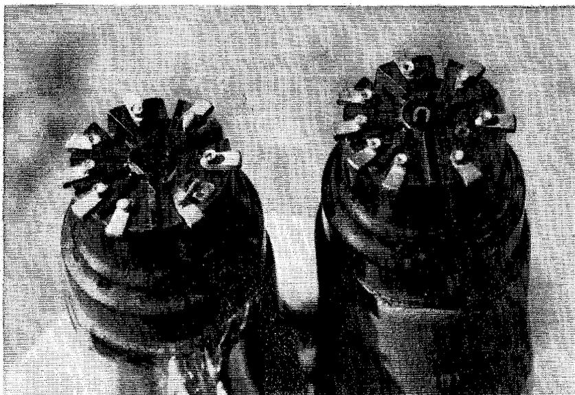
European side contact or P-base valves were produced by some manufacturers from the mid-1930s. P-base valves are most commonly encountered in sets made by Philips and Mullard.
