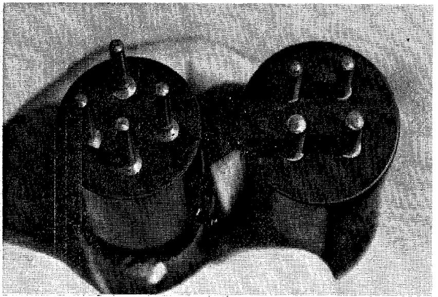
American and European valve bases were of different designs which prevented convenient substitution. At left is the European 4-pin style while at right is the American 4-pin base.
