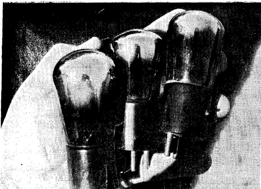
**In the mid 1920s, battery operated triode valves were the only radio valves in common use. Things really were simple in those days!**
