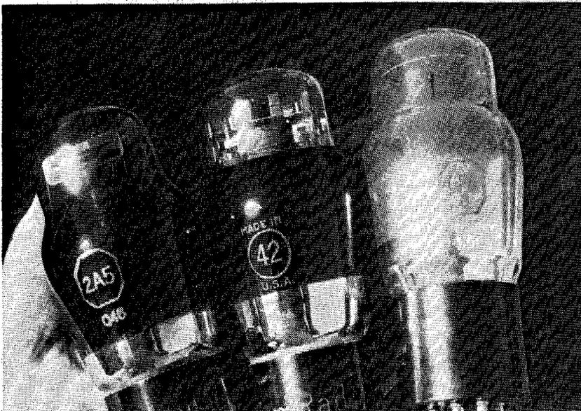
These three valves — 2A5, 42 and 6F6 — have the same electrical characteristics, the only differences being heater voltages and base pin configurations.
