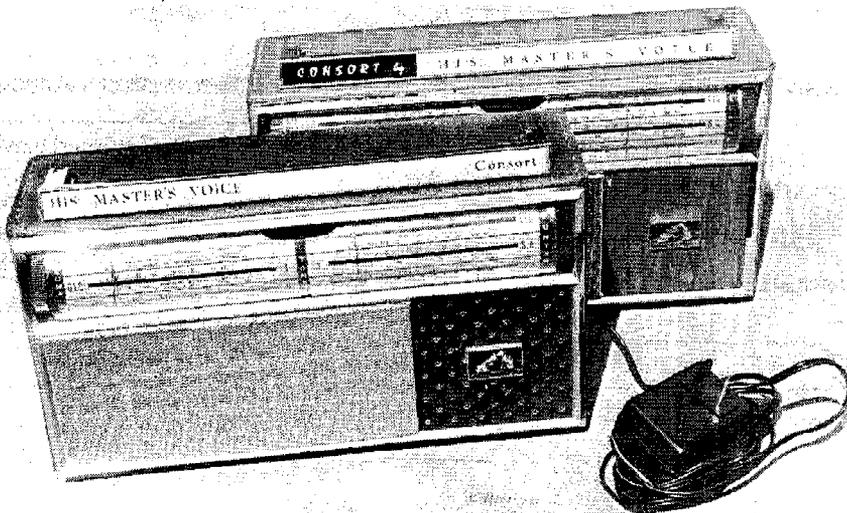
These two old HMV transistor radios are part of the author's collection. The one at the front has been converted to mains operation using a 9V DC adaptor.
