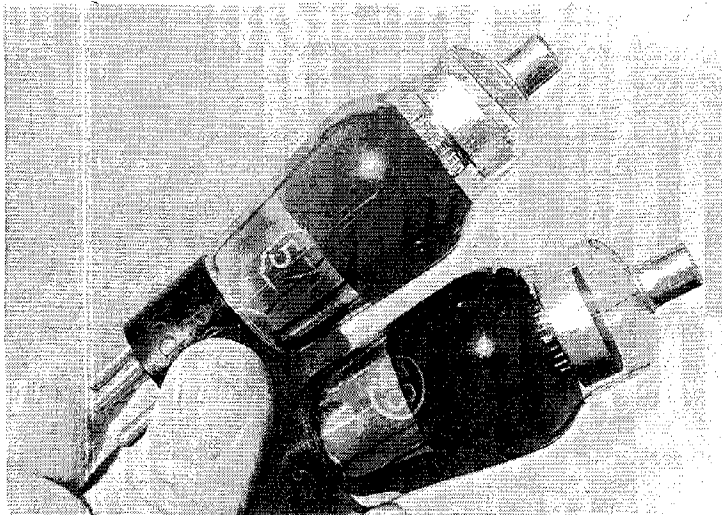
These type 57 & 58 radio frequency pentodes can be used to replace the older type 24 & 35 valves respectively. A new valve socket and minor wiring changes are all that are required. The 57 can also be used in other ways – see text.
