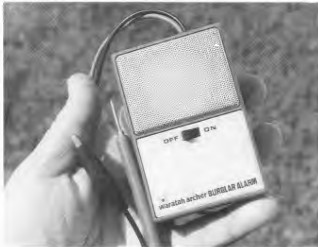
The author's signal injector was built into a convenient cabinet that once housed a low-cost burglar alarm.
