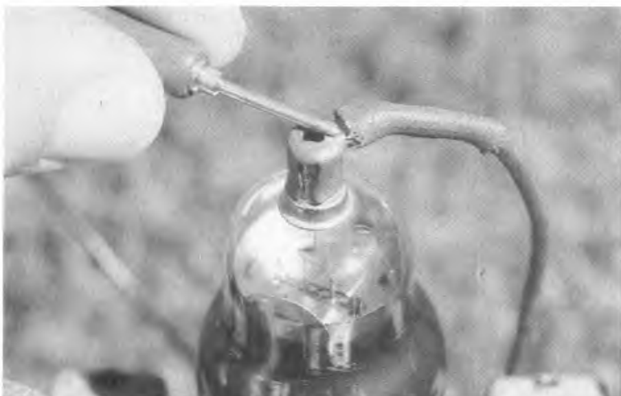
When using the signal injector, the earth clip is connected to the chassis and the probe is connected to the control grid of the valve being tested. A signal injector can quickly locate a faulty stage in a radio receiver.
