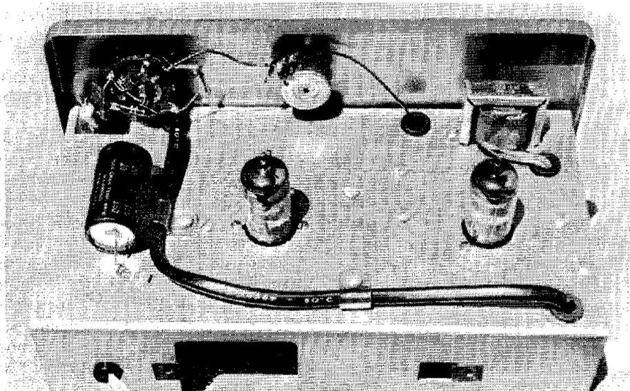
The top of the chassis is neatly laid out and carries the two valves. The Heathkit RF-1 operates from a 110V supply (note the small power transformer) and must be used in conjunction with a 240-110V step-down transformer.
