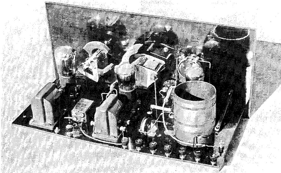
A rear view of receiver after restoration. The wired in "C" battery (two 9V transistor batteries) can be seen between the two audio transformers.
