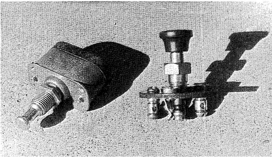
The broken on/off switch (left) was replaced with the switch (right) that was found in the headphone compartment of the cabinet.
