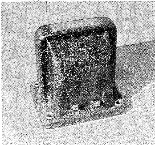
**The defective interstage audio transformer was replaced with a similar unit & the two serviceable transformers then painted to give them a uniform appearance. Open circuit audio transformer primaries are a common problem when restoring a radio of this vintage.**
