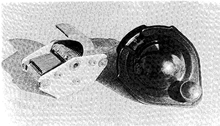
**Cleaning & adjusting the mechanical parts is just as important as servicing the electronic circuitry in a restoration of this nature. This photo shows the restored dial & its companion tuning capacitor.**
