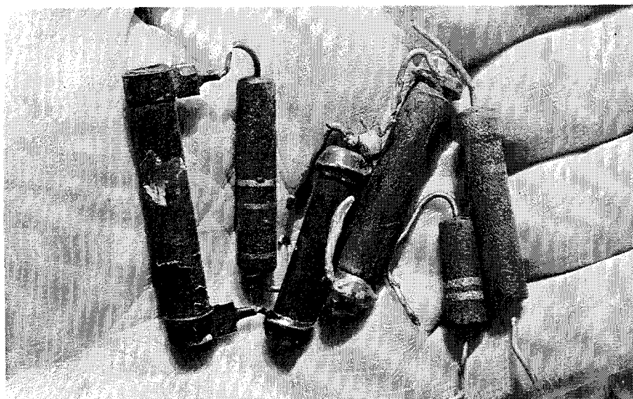
A handful of burnt-out resistors. While a resistor can break down under normal working conditions, an overload caused by a faulty capacitor is usually the cause. Replacing the resistor is pointless unless the real culprit (the leaky capacitor) is also replaced.
