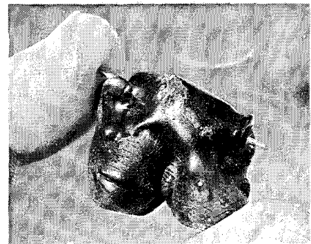
This old capacitor has obviously been running much hotter than its maker originally intended. If a leaky capacitor passes enough current, overheating soon becomes a problem.
