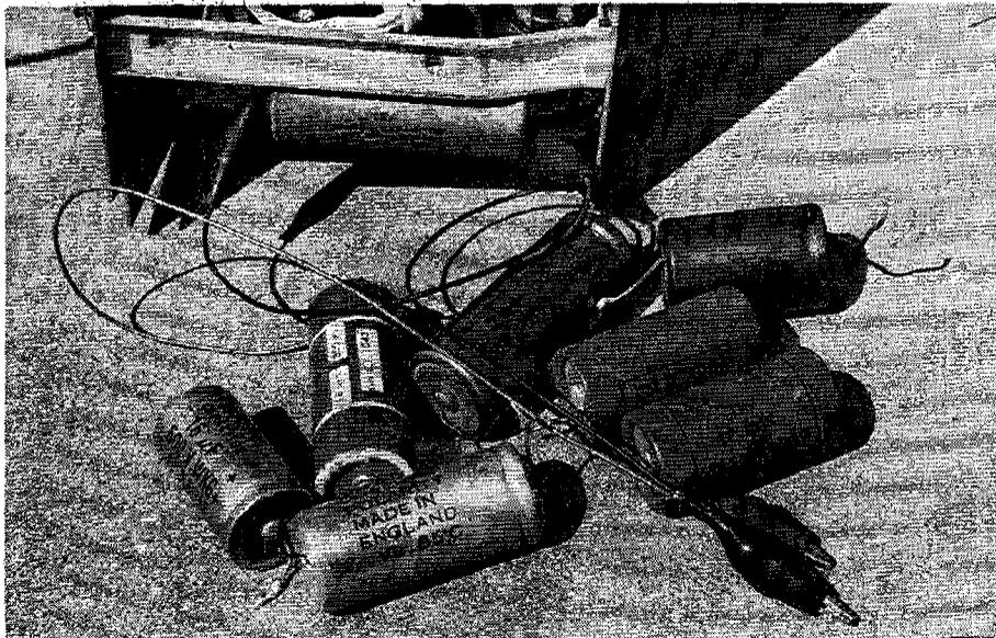
A working chassis can be a convenient high voltage DC supply for checking old electrolytic capacitors. Exercise extreme caution when testing electrolytics in this manner, to avoid receiving a nasty shock.
