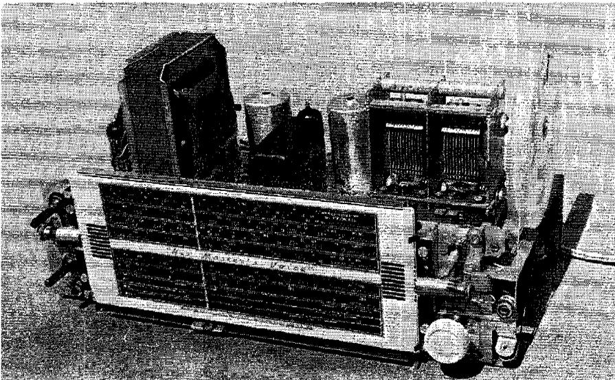
This old HMV radiogram chassis is one of the author's favourite receivers. It has a push-pull output & three shortwave bands. The elaborate glass dial carries all the station call-signs.
