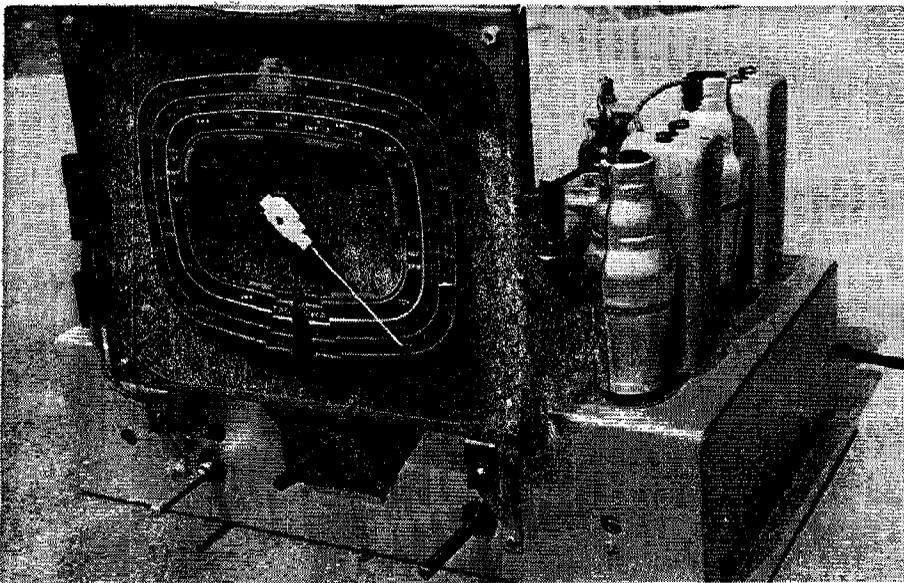
This old chassis is from the early post-war era. It is a 5-valve receiver with shortwave & gives excellent performance when connected to a wall-mounted loudspeaker.
