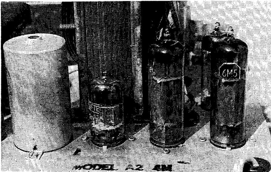
The audio end of the HMV radiogram chassis. It uses a 12AX7 to drive two 6M5 output valves & this arrangement produces more than enough audio power for normal listening.
