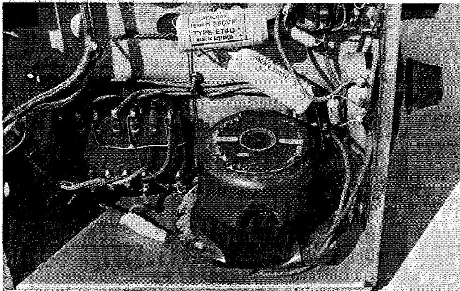
This chassis has been converted for use with a "permag" loudspeaker by fitting the original field coil to one end. Resistors & filter chokes can also be used as substitutes for field coils.
