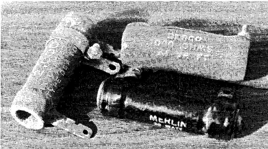
These 20W wirewound resistors can dissipate quite a lot of heat and should be mounted well away from any heat-sensitive components. Note that the resistor on the left is adjustable.
