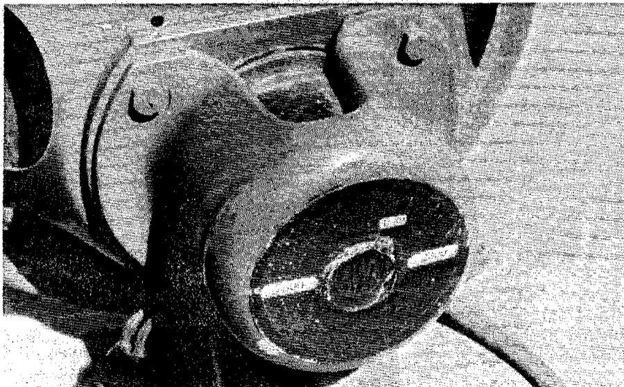
This photo shows the field coil (inside metal housing) of an electrodynamic loudspeaker from the mid-1930s. The field coil played a dual role: (1) it was used as an electromagnet for the loudspeaker; & (2) it was used as a high tension filter choke.
