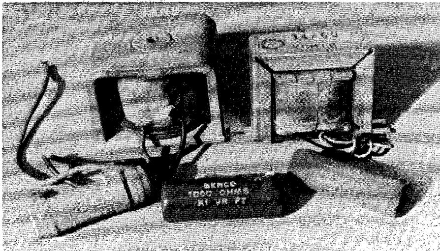
Either a field coil, a choke or a resistor form the central component of most high tension filters. In conjunction with high voltage electrolytic capacitors, they provided adequate H.T. filtering for most valve radio receivers.
