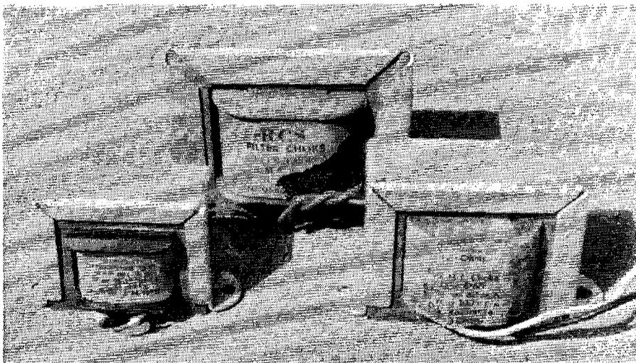
A selection of high tension filter chokes. These chokes perform the same function as a field coil in smoothing the high tension supply & are usually mounted at some convenient spot on the chassis.
