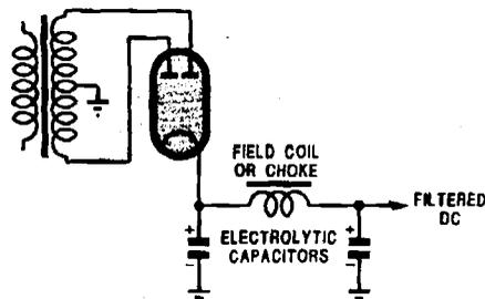
Fig.1: a typical HT power supply for a valve radio receiver. In some circuits, a resistor is used instead of a choke or loudspeaker field coil. HT supplies are a common source of trouble.
