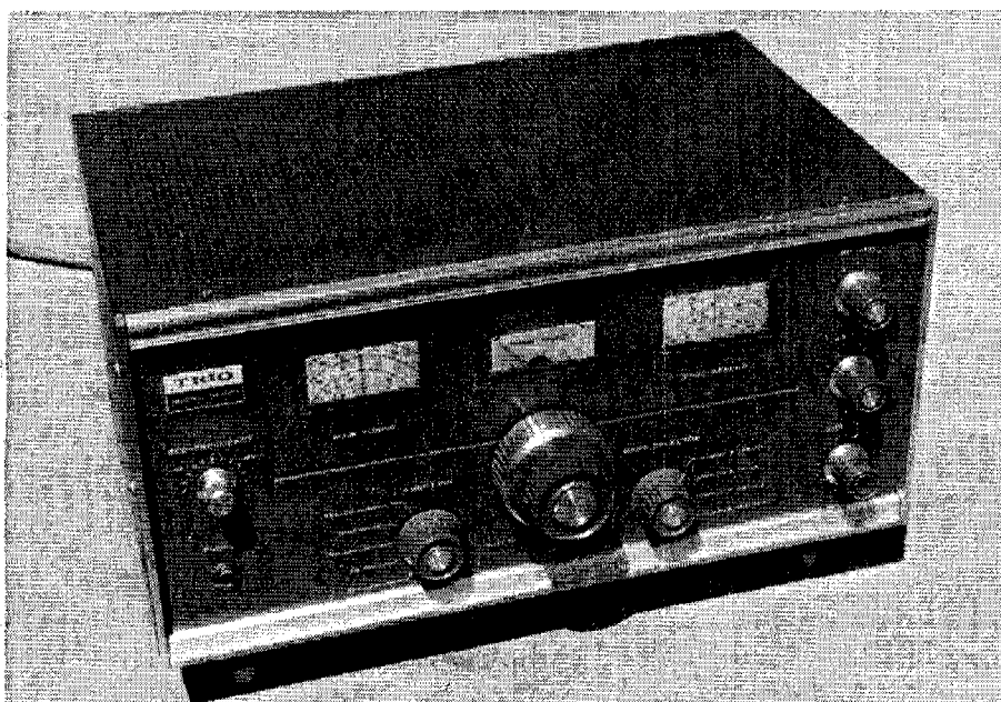
The Trio 9R-59D communications receiver. This particular unit is about 24 years old & although it looked a little unloved when first acquired, the set cleaned up rather well.
