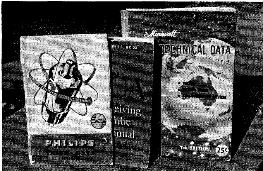
Valve data manuals are invaluable when it comes to substituting valves. These manuals contain details of various valve types & show their socket connections.
