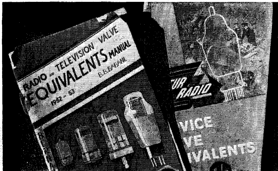
Equivalent manuals are also handy guides when looking for substitute valves. An equivalent valve is one that will fit into the socket & work without modifications to the circuit. A substitute valve, on the other hand, may require extensive socket rewiring or even the fitting of another type of socket.
