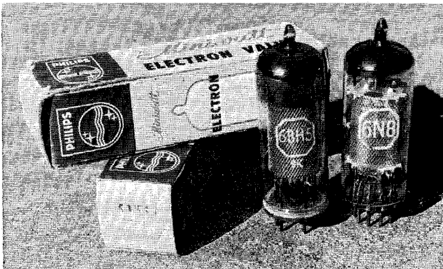
These are the two valves mentioned in the text: the 6BH5 & the 6N8. While both valves can be used as intermediate frequency (IF) amplifiers, they require slightly different socket connections. In the case of the Philips set, someone's failure to make the necessary modifications resulted in a distorted output.
