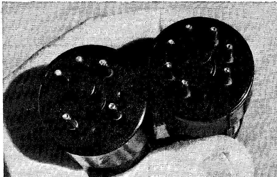
Many valves use only some of their base connections. For example, the 5Y3 (left) has just 5 pins, while the 6V6 (right) has 6 or 7 pins. Receiver manufacturers often used vacant socket terminals as convenient mounting points for other components & so a substitute valve may require considerable socket rewiring.
