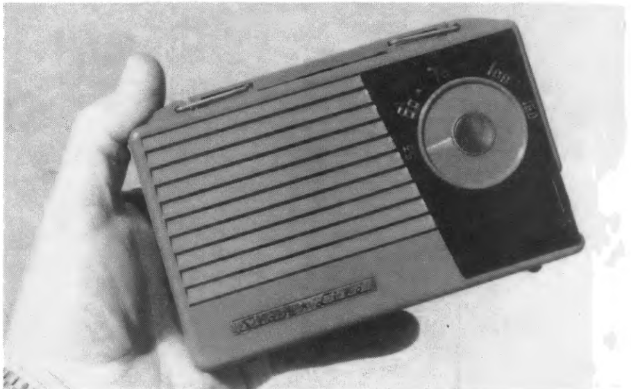
The Japanese-made Starlight pocket portable was similar in appearance to later-model transistor radios. It featured a combined volume on/off control, a direct drive dial, a carry handle & an earphone socket.
