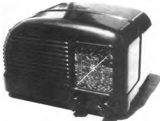
The STC Bantam is unique in that it is a very small radio that was been built using full sized components. Like the Philips set it is a full superhet design & is a good performer.
