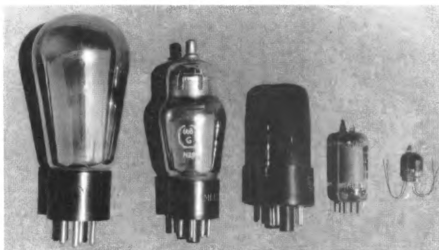
Over the years, valves diminished in size to quite a remarkable degree. This view shows, from left, a 45, 6G8, 6V6, 6BE6 & a Z70U. The latter is a truly miniature triode.
