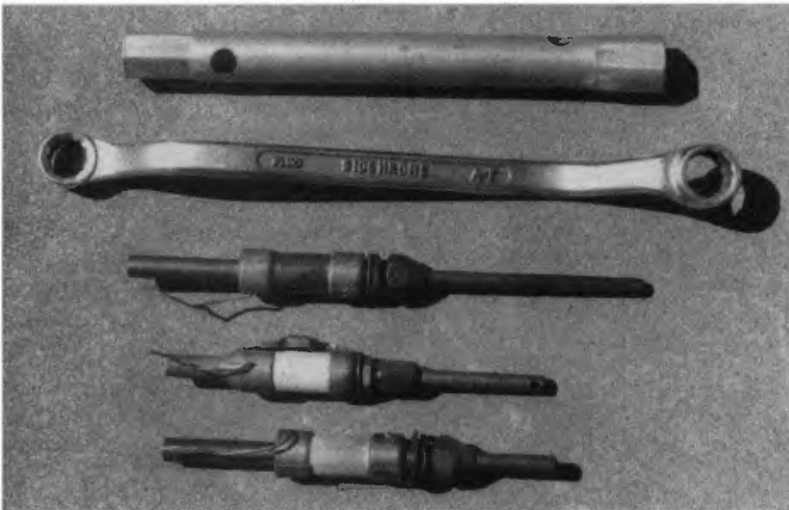
Tube & ring spanners are handy when adjusting some of the trimmer capacitors found on old radio sets. While these trimmers may be awkward to adjust, once set they stay that way.
