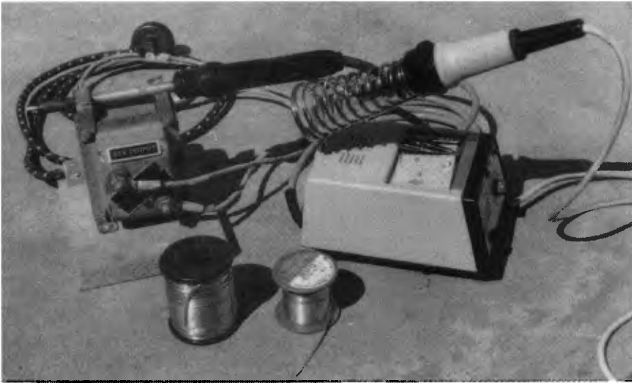
These two soldering irons can handle just about any vintage radio soldering job. They include an old-style Scope soldering iron & transformer (left) & a modern temperature controlled iron.
