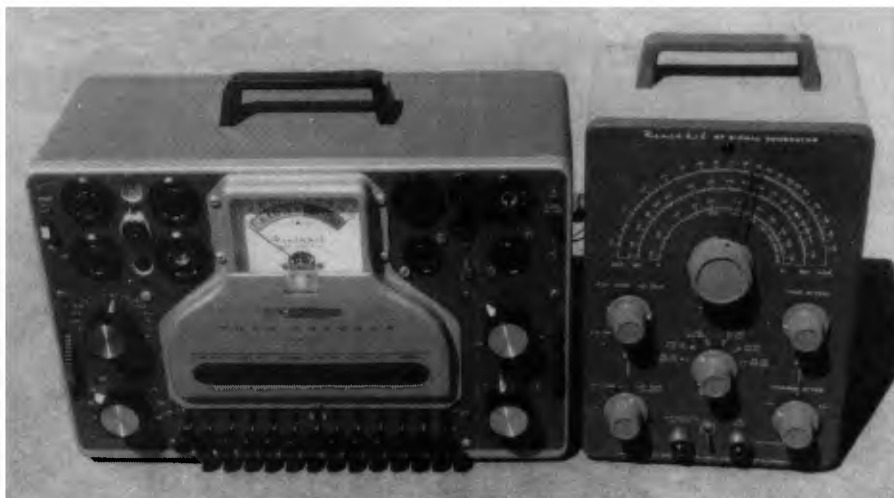
This photo shows the author's valve tester & radio frequency (RF) generator, both of which were originally built from kits. Valve testers are hard to come by these days, although RF generators can be readily purchased from electronics retailers.
