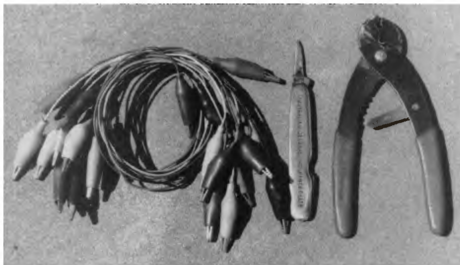
This basic equipment for the workbench includes several sets of jumper leads, a small pocket knife & a pair of wire strippers.
