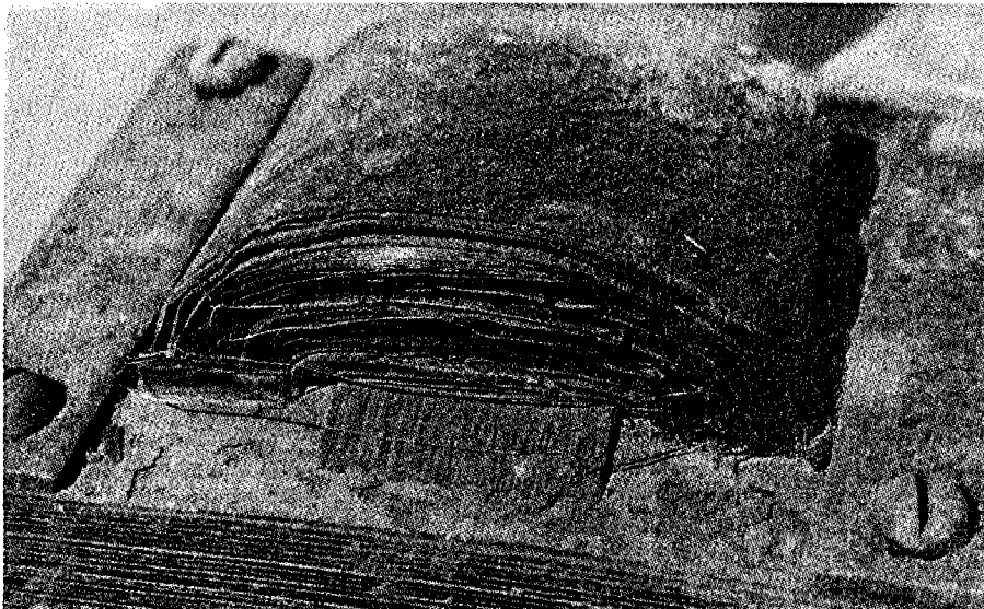
The power transformers used in many Philips & Mullard receivers share this common fault – an exposed high tension winding. The winding protrudes outside the paper insulation that separates the layers (probably caused by the paper shrinking with age). This is not the transformer used in the Philipsette in the story but a similar one in worse condition, to show the problem more clearly.
