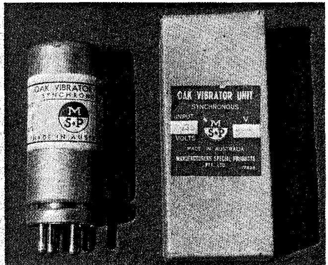
A new 4V vibrator unit to suit the Radiola was unearthed in the author's miscellaneous parts cupboard. Vibrators of this type would be rare items today as they went out of use with the advent of the transistor radio.
