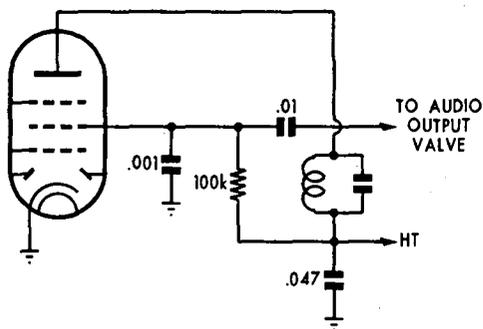
**Fig.3: in some reflex sets, the audio is taken from the screen of the audio valve instead of from the plate. This circuit shows the basic scheme.**
