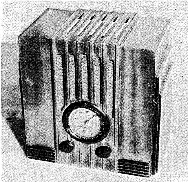
This timber cabinet Radiola Model 27 was the first of the Radiolette series to use a reflex circuit. Reflex receivers were common throughout the 1920s, 1930s and 1940s and were particularly popular in Australia.
