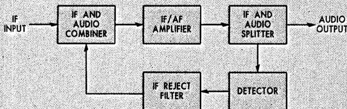
Fig.1: block diagram of a reflexed radio receiver. The reflexed valve has a signal combiner at its input which combines the IF and audio signals, the combined signal then being fed to the valve for amplification.
