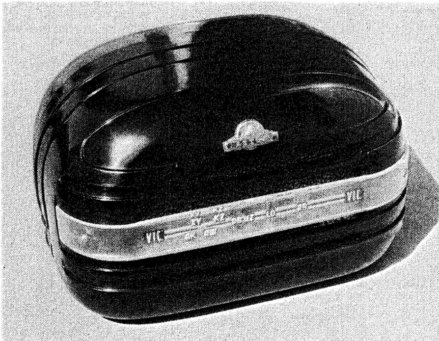
The Astor "Football" was a 3-valve reflexed TRF receiver. The 6B8-G valve in the little Astor provided RF and AF amplification plus detection, so it was quite a busy little valve.
