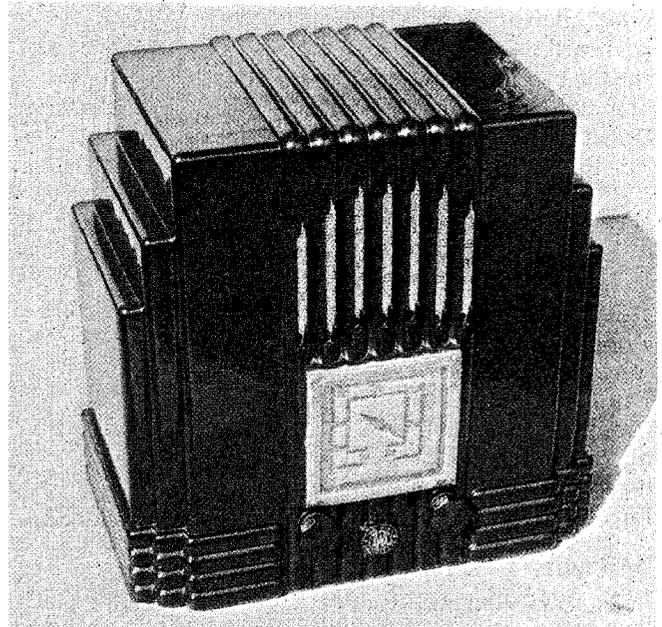
Another reflexed Radiolette receiver. Reflexing gave a receiver a substantial performance lift without the expense of adding another valve but the circuit had to be carefully designed.
