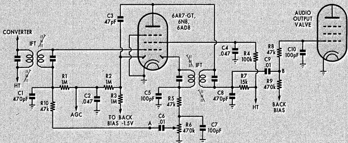
Fig.2: a practical reflex circuit. The valve used was often a 6AR7-GT in the octal days, while the 6N8 and 6AD8 were used more in the miniature days
