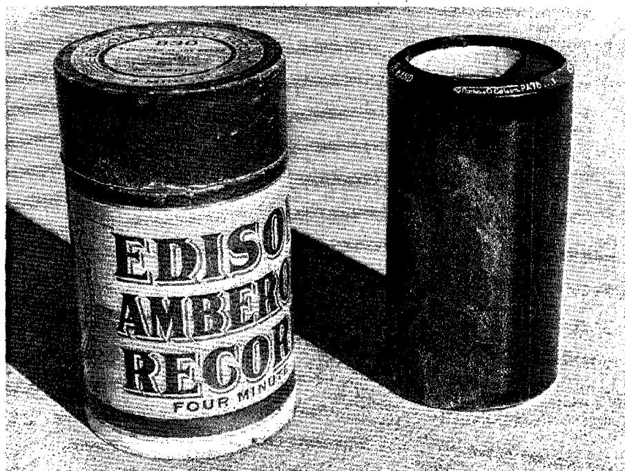
A genuine four-minute Edison cylindrical record. These early records were "hill and dale" types; ie, the modulation of the groove was up and down, not sideways as in later years.
