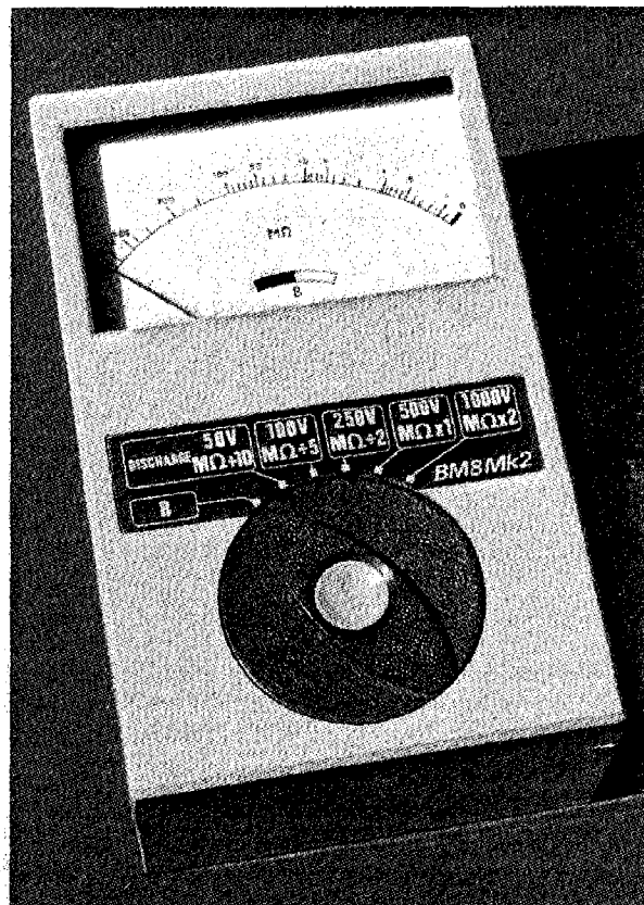
Right: a modern electronic Megger. Gone is the old crank handle used in early design to generate the test voltage. The trademark is faintly visible at right, just below the meter scale.
