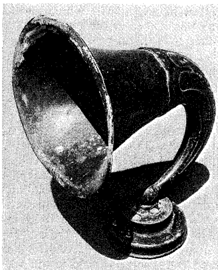
This Brown horn speaker is one of the better types in that it has an aluminium cone instead of the usual soft iron diaphragm. Its tonal qualities and sensitivity were better than most.
