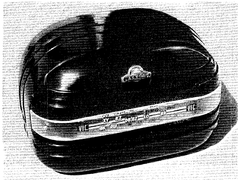
The 1948 GR model Baby Astor was known to collectors as the Astor "Football". It is a 3-valve reflexed TRF receiver of fairly limited performance.
