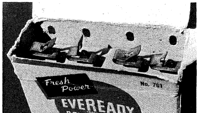
This old Eveready "C" battery contains three size "D" cells wired in series. The close-up view (above) shows the battery connections. The terminals, from left to right, are 0V, -1.5V, -3V and -4.5V.
